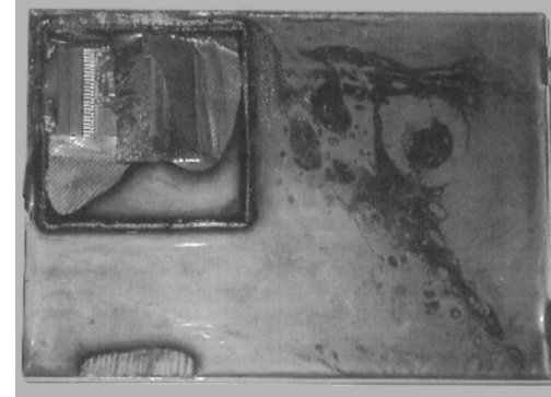
Tamper mesh from the IBM 4758 cryptoprocessor
